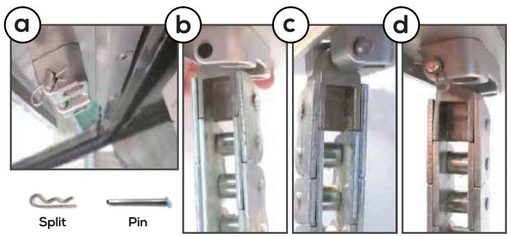
a. Remove split and pin from the chain bracket.
