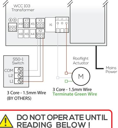
Engaging the actuator before reading the next page will damage rooflight.
