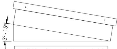
Rooflight must be installed on a roof pitch between 3-30° (by others). Failure to do so will result in water pooling on the rooflight.
