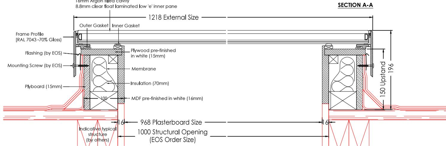
3-30 degree pitch must be on smaller size if modular rooflight has an opener as motor must sit level and not on a pitch.
