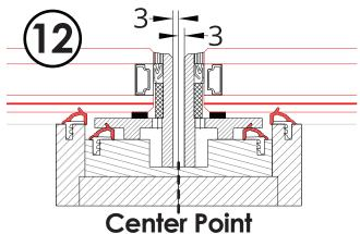
12. Use center mark to check placement and that the rooflight is central.
