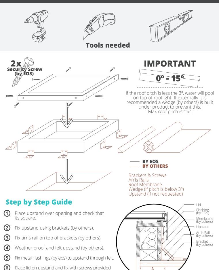
Place lid on upstand and fix with screws provided (security screws should be on opposite sides).
